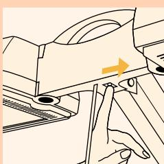
► The measuring tape will automatically rewind if you move the red tab sideways.
