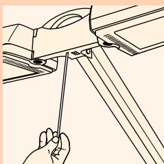
► You can determine whether the appliance has been set to the required height by pulling out the measuring tape.
